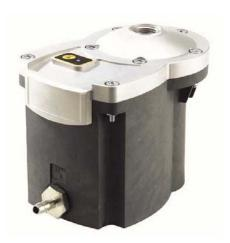
The **Enterprize** Zero Air Loss Drain from PREMIER uses an innovative combination of software with transducer interface to continuously measure the presence of condensate - ensuring no loss of compressed air. Constant monitoring of condensate volume within the drain, at a rate of 50 times per second, results in the fast and effective discharge of up to 80 gallons of condensate per hour. It operates equally well with clean, heavily emulsified, and dirty condensate.
